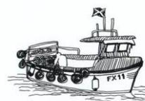
This is a **prawn trawler**; the gear is normally stowed on deck at the stern; there is a large bow wave. When fishing they would be moving slowly – about 2-3 knots; a leisurely walking pace. The lines to the net are usually over the stern or close in to the sides. These boats work the deeper muddy sea floor.
